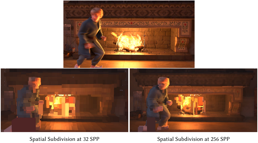
Fig. 7. A rendering from Frozen 2 and the corresponding voxel representation of the spatial subdivision at 32 and 256 samples per pixel. © 2025 Disney
