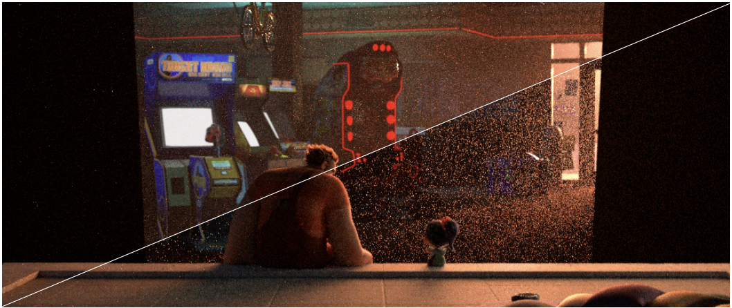
(a) Rendered without path simplification. With path guiding (top left) and without path guiding enabled (bottom right).
